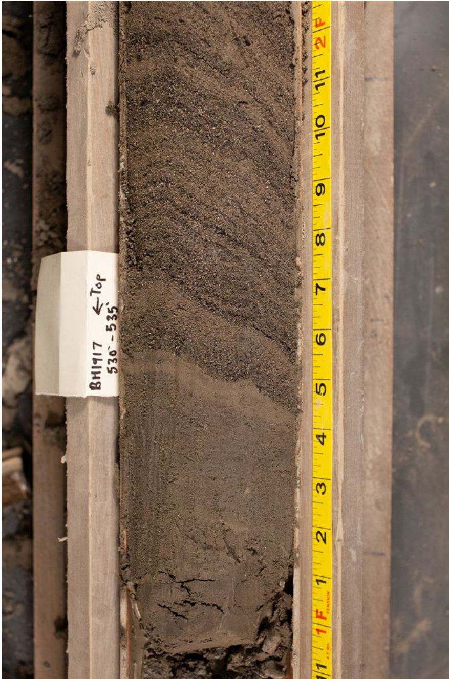
Figure 1. Recovered PQ-wireline core of bedded sand unit; note original bedding and minimal disturbance of original sedimentary structures.
